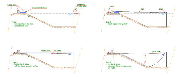
Figure 12. Sequence of submerging the geomembrane (Genap BV, 2015)
